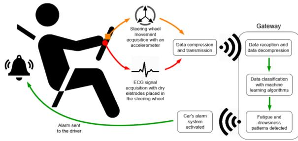
Figure 2: Block diagram of the proposed system (left) and its placement on the automobile (right).
